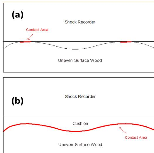
**Figure 4:** (a) Shock Recorder Placed on Pallet Top Board without Cushion; (b) Shock Recorder Placed on Pallet Top Board with Cushion
