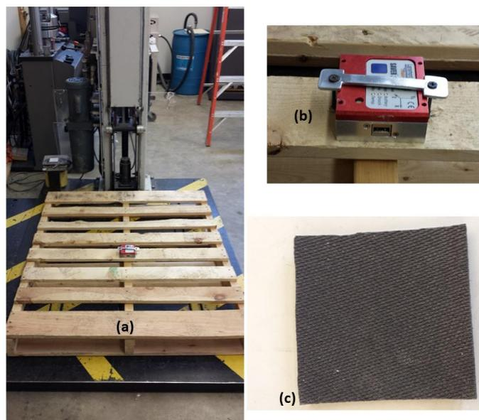
**Figure 1:** (a) Pallet on Drop Tester, (b) Shock Recorder, and (c) Anti-Vibration Pad
