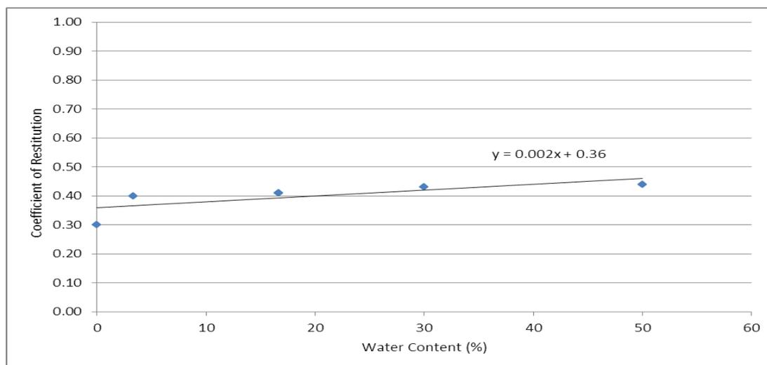
**Figure 9:** Result From Experiment 4 – Coefficient of Restitution
