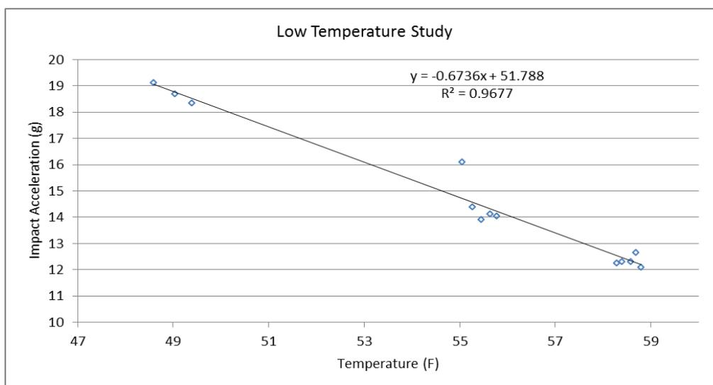
Figure 11: Impact Acceleration vs Temperature (48°F to 59°F)
