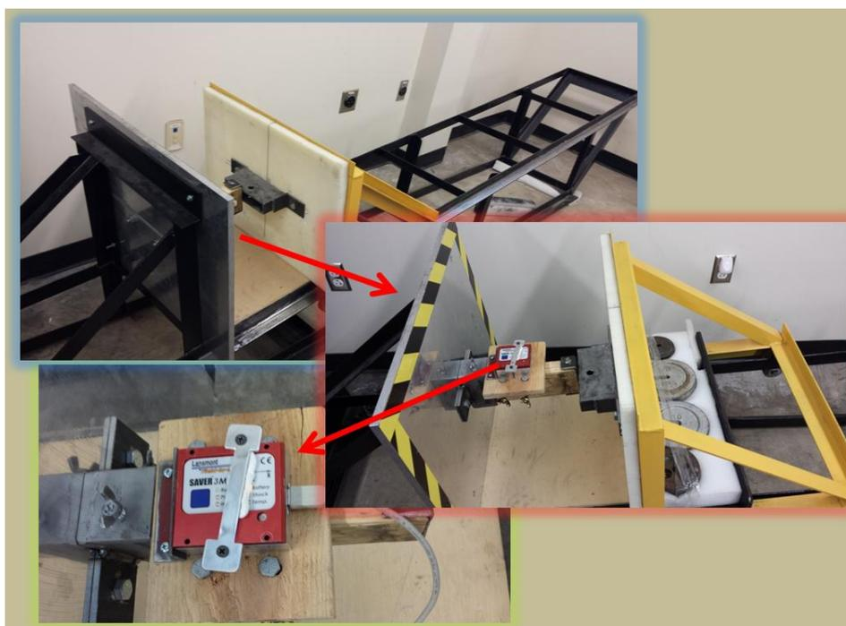
*Figure 7: Incline Impact Test Setup*
