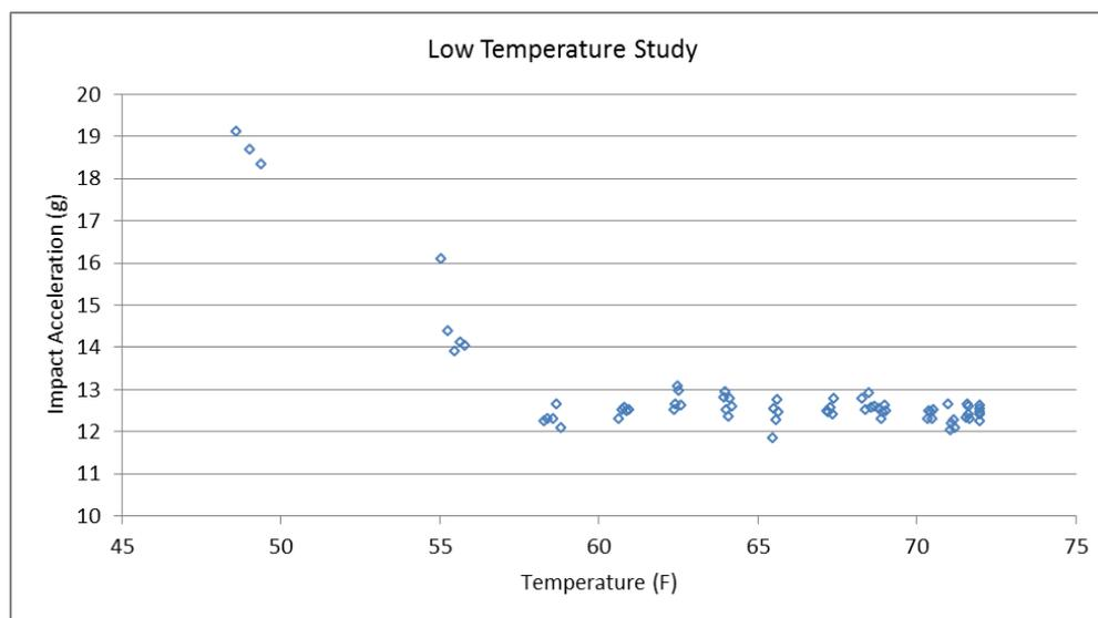
**Figure 10:** Impact Acceleration vs Temperature ( $48^\circ\text{F}$  to  $72^\circ\text{F}$ )
