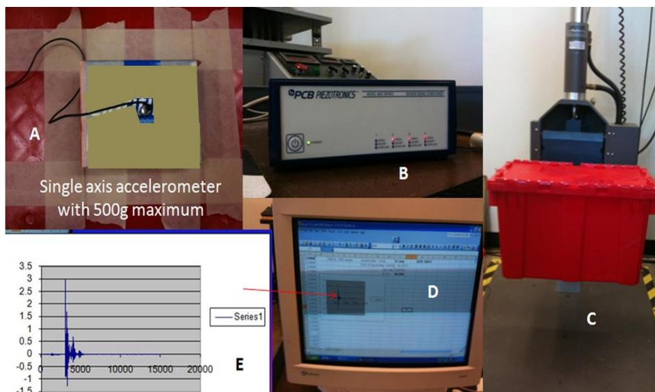
**Figure 5:** Setup for Cushioning at the Tote Bottom
