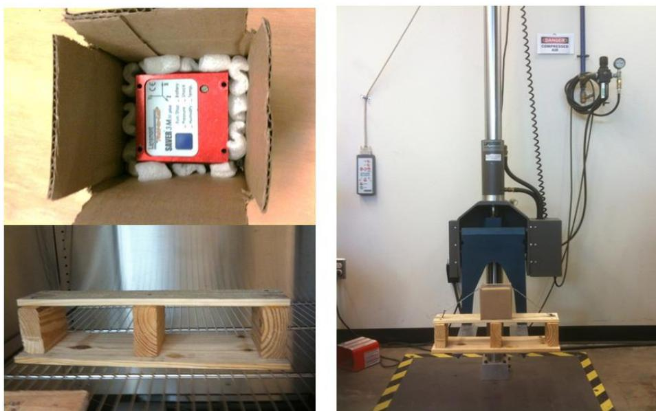
**Figure 6:** Drop Test of Pallet Specimens
