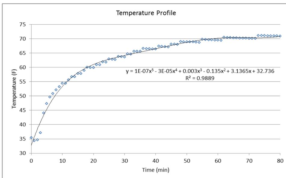
**Figure 4:** Warm-up Curve for Low Temperature Study
