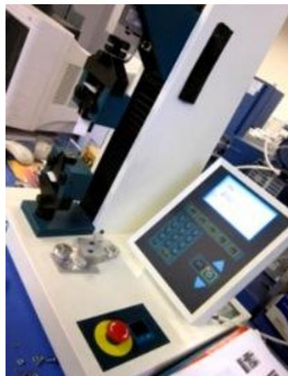
**Figure 2:** H5KS Tensile Tester
