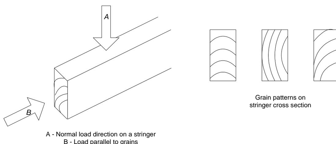
**Figure 1:** Loading Orientations for Static Compression Test
