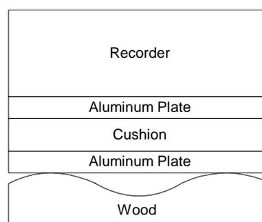
**Figure 6:** Anti-vibration Pad Placed Between Two Aluminum Plates (Case 5)
