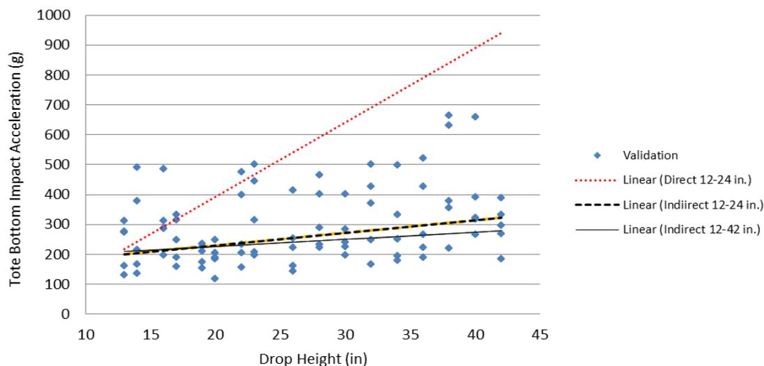
**Figure 11:** Validation of Tote Bottom Impact Acceleration
