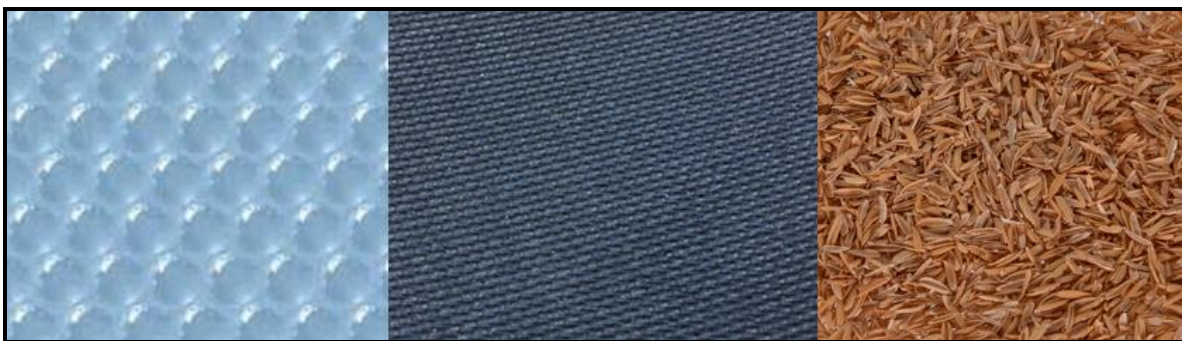
Figure 1: Cushioning Materials Used in This Study: 3/16-inch Bubble Wrap (left), 0.129-inch Thick Anti-Vibration Pad (center); and Rice Hulls (right)
