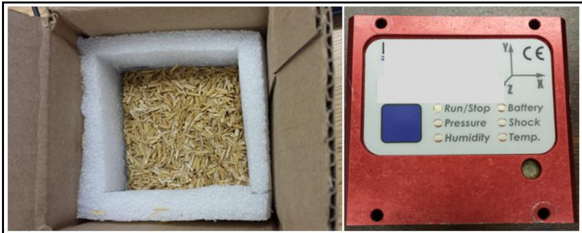
Figure 2: Shock Recorder Setup
