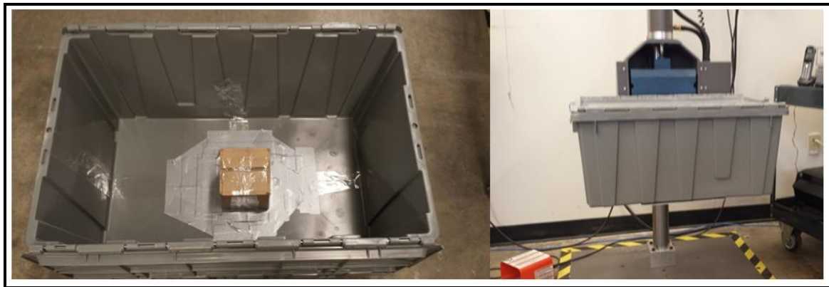
Figure 3: Plastic Tote and Drop Test
