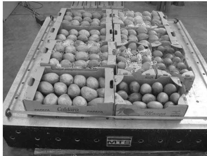
Figure 2: Disposal of Packaging on a Vibration Table
