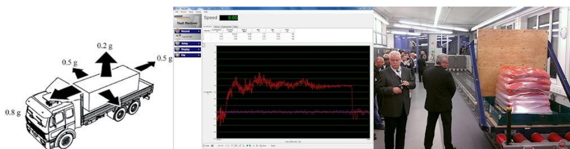
Figure 4: (a) Typical Forces Experienced Due to Braking, Accelerating and Turning , (b) Load Stability Test System Installed at Fraunhofer Institute in Dortmund, Germany
