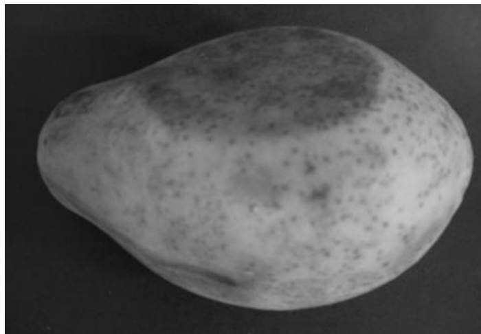
Figure 4: Papaya with Serious Damage – System with No Cushioning
