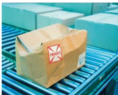
Figure 1: Damaged Corrugated Container Due to Reduction in Structural Material Used
