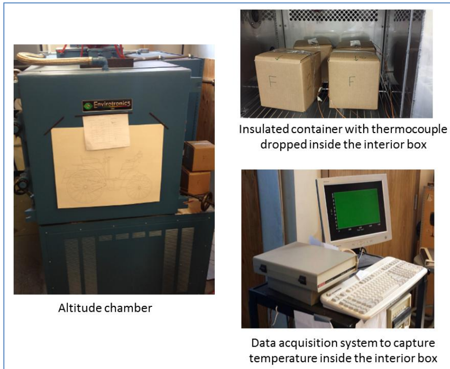
Figure 2: Insulated Container, Altitude Chamber, Thermocouple, and Data Acquisition System
