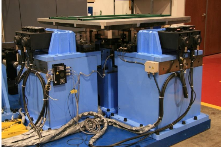
Figure 2: Kokusai, Inc. three-axis electric servo motor vibration table
