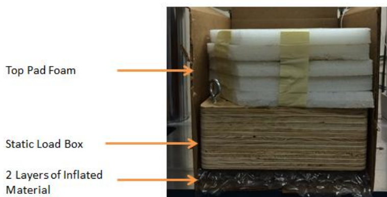
Figure 2: Example test setup used for the cushion system
