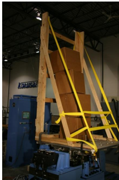
Figure 15: Single stack instability as a result of simultaneous multi-axis vibration
