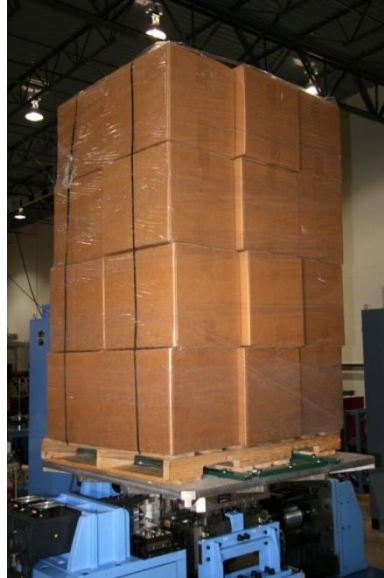
Figure 14: Unit load instability as a result of three minutes of simultaneous multi-axis vibration
