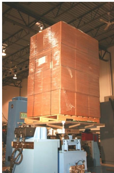
Figure 5: Unit load stability test setup
