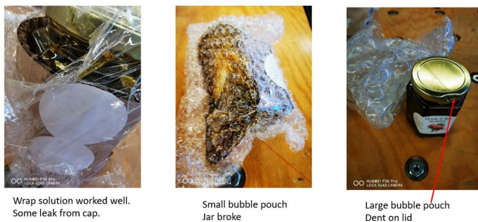
Figure 13: Damages of 12-oz Honey Jar from 30-Inch Drop
