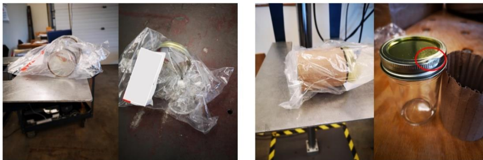
Figure 10: Preliminary Drop Test of Similar Glass Jars
