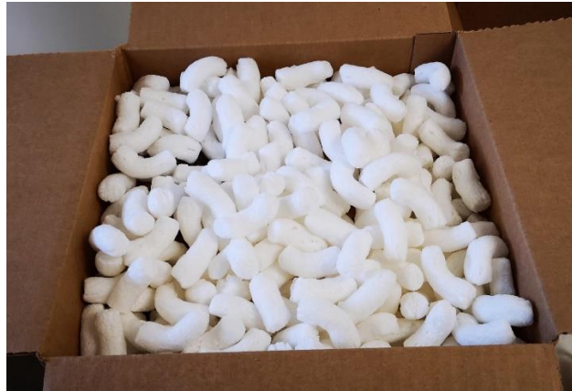
Figure 9: Biodegradable Peanuts as Filler and Cushioning Material
