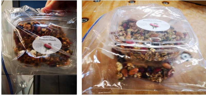
Figure 12: 48-inch Side Drop of Granola Tray Caused Lid Popping
