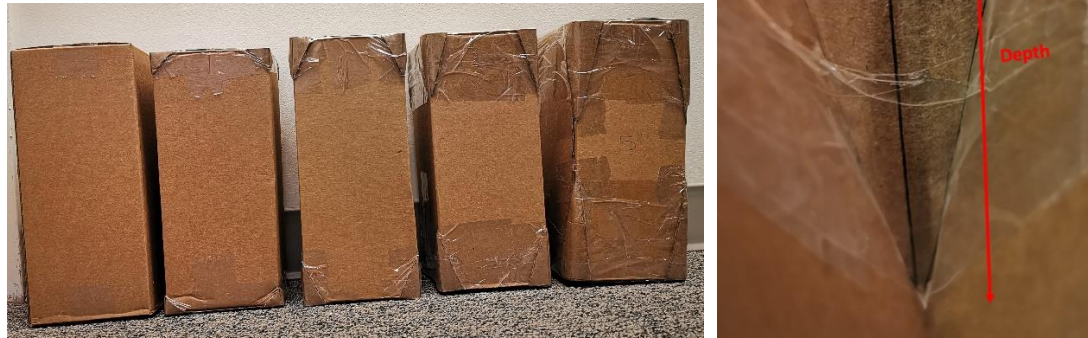
Figure 8: Triangular Corner Stiffeners with Various Depths
