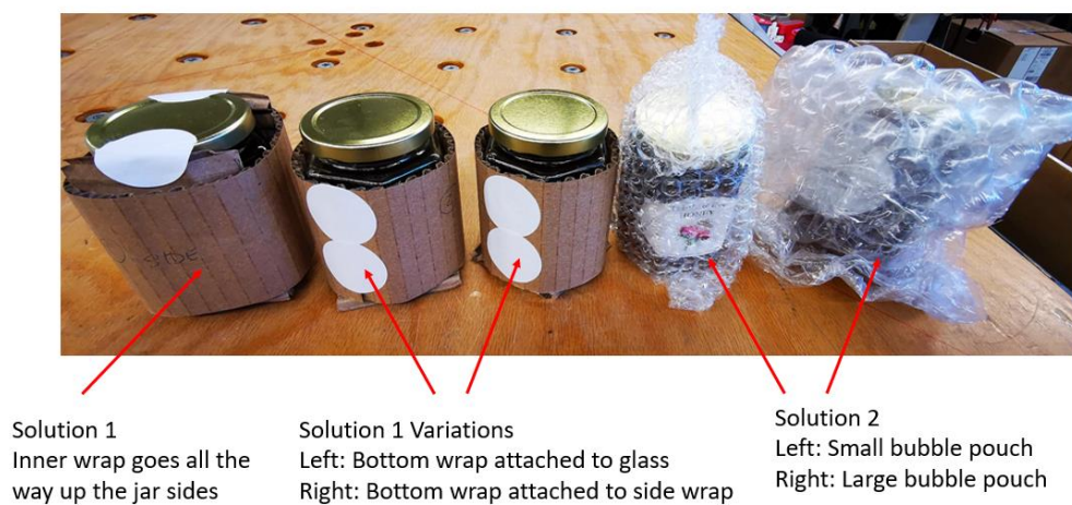
Figure 12: Various Solutions to Protect 12-oz Honey Jar from Breakage of 30-Inch Drop
