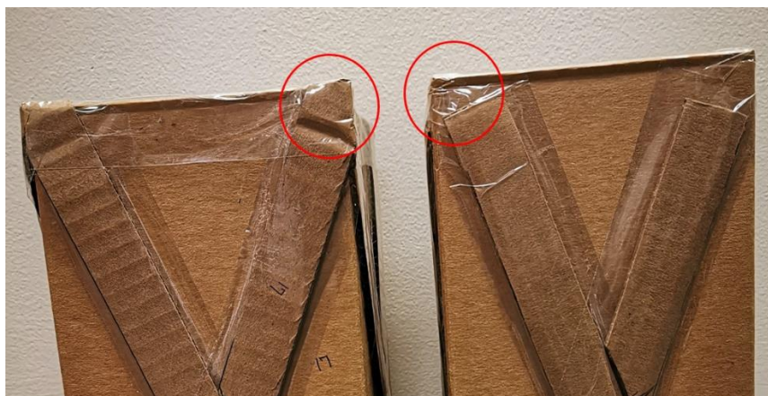
Figure 6: Corner-Fitting Brace (Left) vs Corner-Unfitting Brace (Right)
