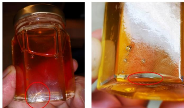
Figure 11: 3-oz Honey Jar with Single-Face Corrugated Wrap: 48-Inch Drop (Left) & 30-Inch Drop (Right)
