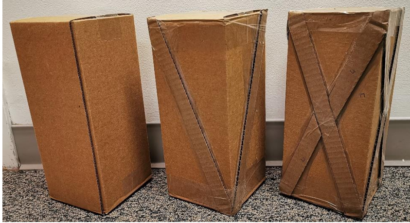
Figure 5: Single and Cross Diagonal Braces.
