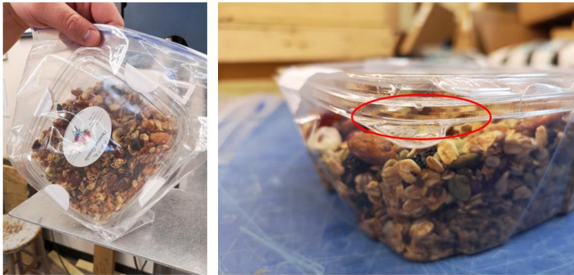
Figure 13: 48-inch Corner Drop of Granola Tray with Lid Secured by Four Paper Labels
