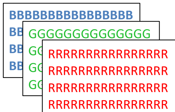
Figure 8: RGB pixel values are stored in the form of a 3-D matrix
