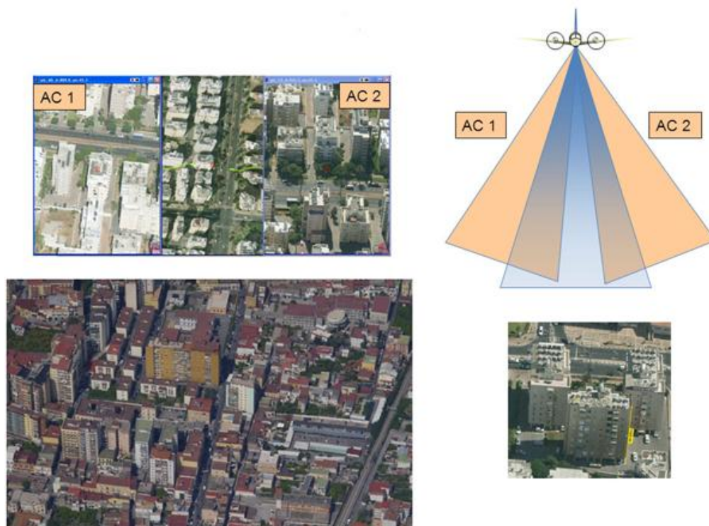
Figure 1: Oblique Sensors Integrated into the Process of Photogrammetric Surveys
