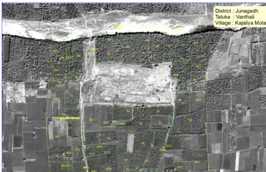
Figure 10: CARTOSAT-1 image with survey numbers having fruit crop plantations in Vanthali Taluka
