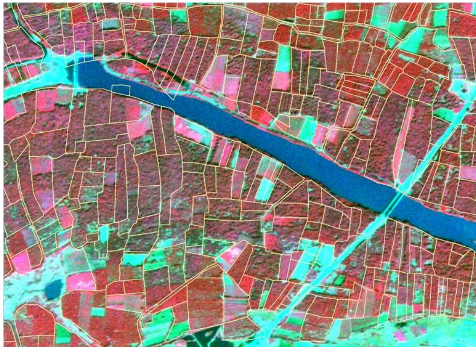
Figure 7: IRS LISS-IV image of Vanthali village with plot boundaries superimposed from cadastral maps
