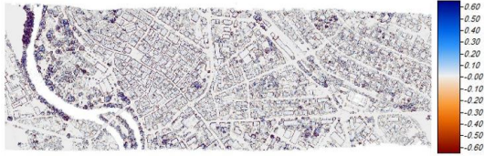
Figure 3: Feature Layer extracted from LiDAR DSM using Gaussian low pass filter of 3x3 window size
