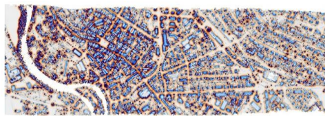
Figure 7: Feature Layer extracted from LiDAR DSM using low pass Gaussian filter of 31x31 window size
