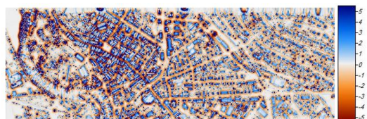
Figure 13: Feature Layer extracted from LiDAR DSM using focal analysis mean filter of 31x31 window size
