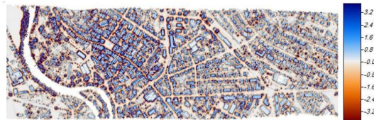
Figure 6: Feature Layer extracted from LiDAR DSM using Gaussian low pass filter of 21x21 window size
