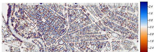
Figure 11: Feature Layer extracted from LiDAR DSM using focal analysis mean filter of 11x11 window size
