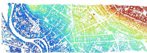
Figure 15: Feature layer extracted from LiDAR DSM with the use of DTM slope-based filter of 3x3 window size
