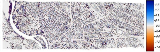
Figure 4: Feature Layer extracted from LiDAR DSM using Gaussian low pass filter of 7x7 window size
