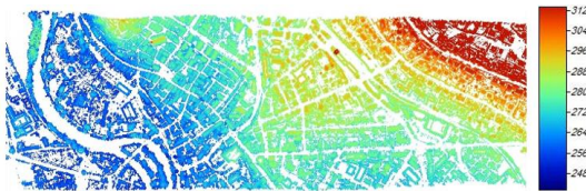
Figure 18: Feature layer extracted from LiDAR DSM with the use of DTM slope-based filter of 21x21 window size
