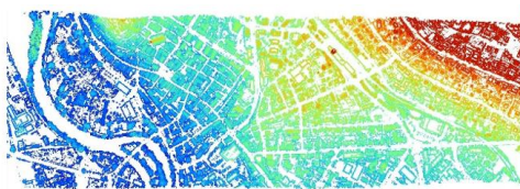
Figure 17: Feature layer extracted from LiDAR DSM with the use of DTM slope-based filter of 11x11 window size
