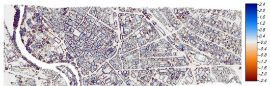
Figure 5: Feature Layer extracted from LiDAR DSM using Gaussian low pass filter of 11x11 window size
