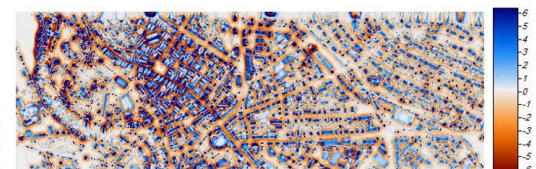
Figure 14: Feature Layer extracted from LiDAR DSM using focal analysis mean filter of 41x41 window size
