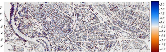
Figure 10: Feature Layer extracted from LiDAR DSM using focal analysis mean filter of 7x7 window size
