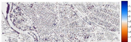
Figure 9: Feature Layer extracted from LiDAR DSM using focal analysis mean filter of 3x3 window size
