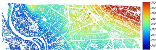
Figure 16: Feature layer extracted from LiDAR DSM with the use of DTM slope-based filter of 7x7 window size
