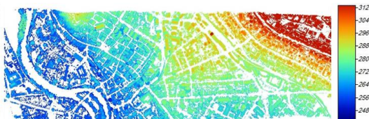
Figure 20: Feature layer extracted from LiDAR DSM with the use of DTM slope-based filter of 41x41 window size
